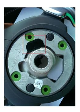
2. Drill a hole (red mark on picture below) and screw a bolt
