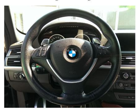
1. Remove airbag – detach mechanical latches (can be done with flat screwdriver)
