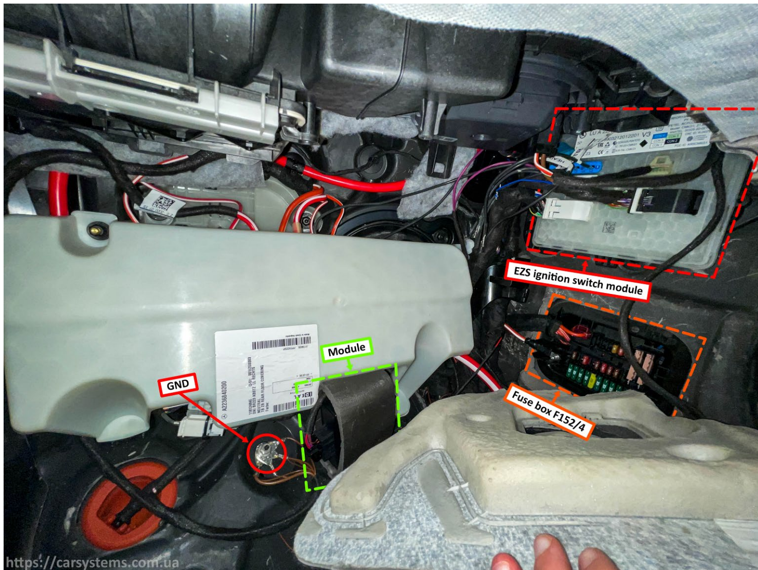
Picture 2 Elements location for Module installation
